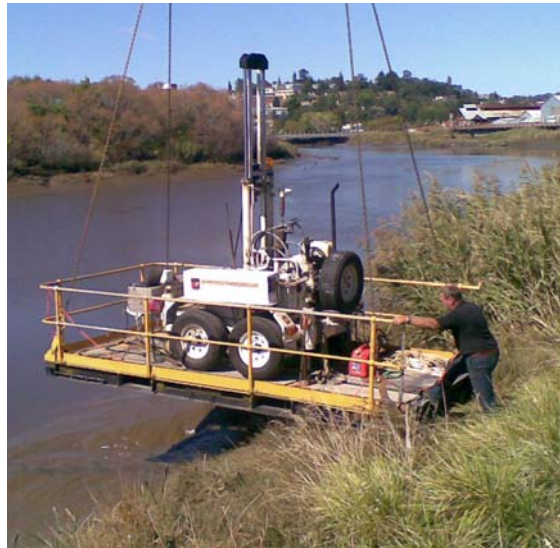
Figure 9. CPT testing on river levee, Launceston (Courtesy Pitt & Sherry, TAS).
