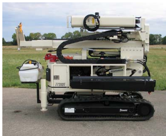
Figure 10. Geoprobe Geo7720DT tracked CPT drilling-sampling rig (US), operated with Geotech AB (Sweden) cordless CPT probes (Courtesy Brown Bros Ltd, www.brownbro.co.nz )
