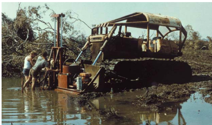
Figure 1. CPT testing in the 'mangrove swamp' at the mouth of the Brisbane River for the SI for Brisbane Airport, 1980, showing the CPT rig attached to the blade of a Komatsu bulldozer (photograph courtesy of Allan McConnell, IGS, http://www.insitu.com.au/ )
