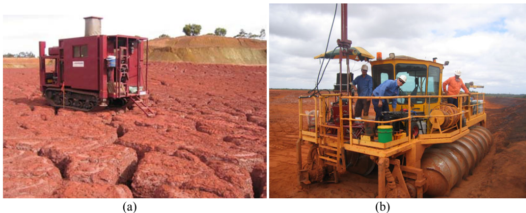
Figure 8. (a) Marooka 12t tracked CPT rig operating on tailings storage with desiccated crust, Kalgoorlie, WA; and (b) portable CPT rig set up on an “Amphiroll” vehicle on a bauxite residue (‘red mud’) tailings storage area, Kwinana, WA (Courtesy of Probedrill: www.probedrill.com.au ).
