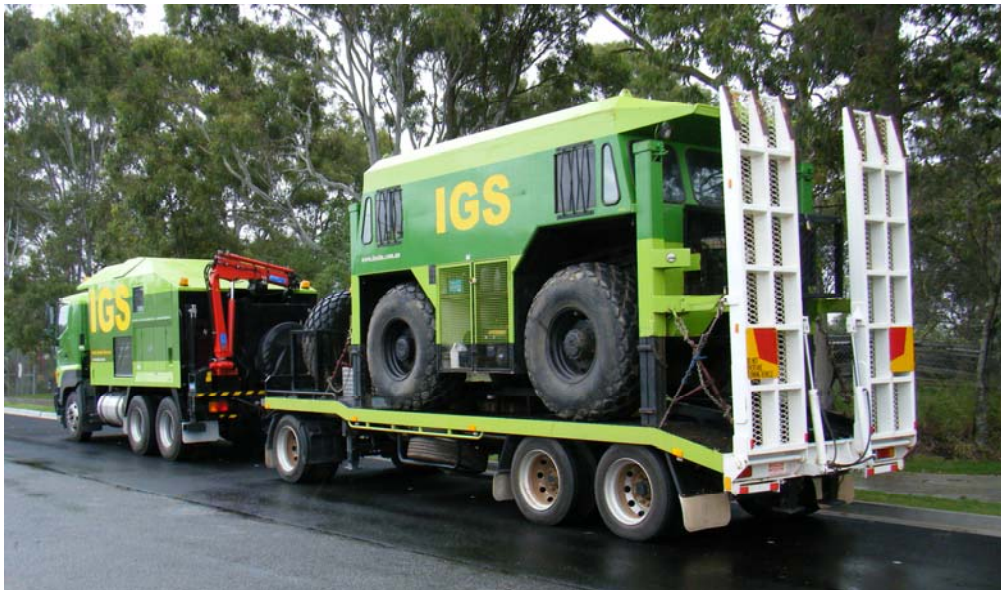
Figure 5. Mobilising two CPT trucks: a 20t 6×4 rig set up to haul a trailer with a 10-20t all-terrain rig (Courtesy Allan McConnell, IGS, http://www.insitu.com.au/ )
