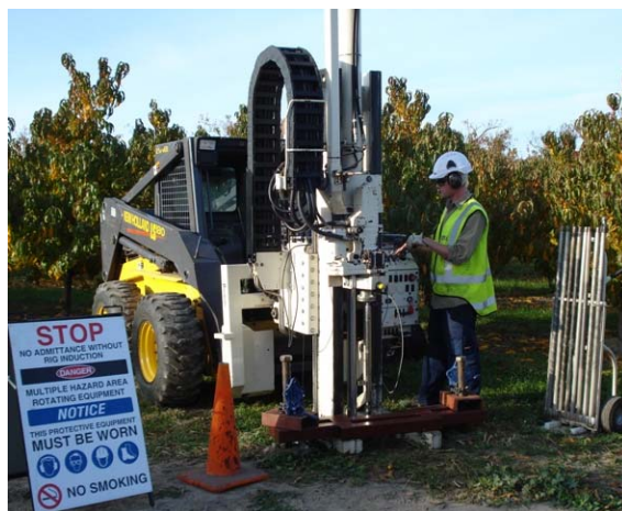
Figure 11. CPT rig on New Holland LS180 Skid Steer; reaction provided by ground anchors (RDCL, NZ, www.rdcl.co.nz )
