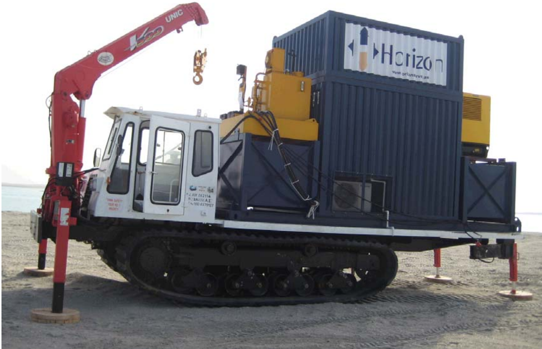
Figure 2. A photograph showing a track-mounted CPT rig used in Dubai, UAE.
