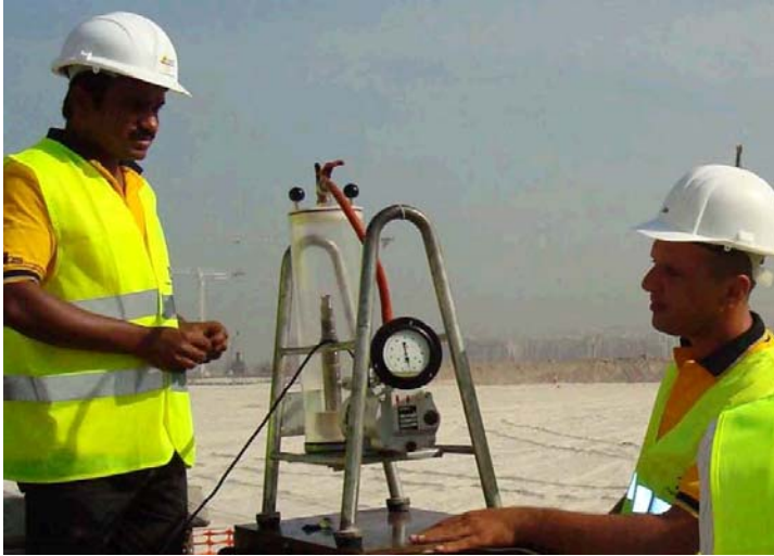
Figure 3. A photograph showing the saturation of Piezo-cone in Dubai, UAE following the IRTP procedure.
