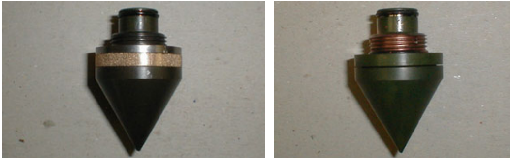
Figure 4. Cone tips with porous filter of sintered bronze (left) and slot filter (right) ( www.envi.se ).
