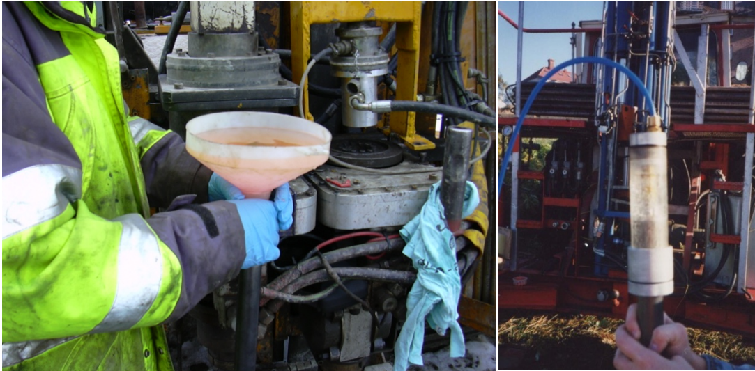
Figure 3. Saturation of the CPTU probe with a) Submerged mounting and b) Vacuum treatment.
